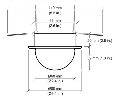
Measurements in millimeters and inches (in brackets).
