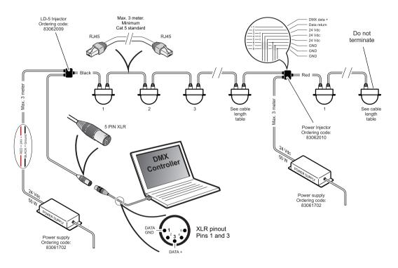
A single power supply can drive multiple LD-5s, but note that the strength of the current falls between each LD-5 and the degree of this drop is also dependent on the length of the cable. The following table provides some guidelines, but for additional guidance, contact SGM or your local distributor.
